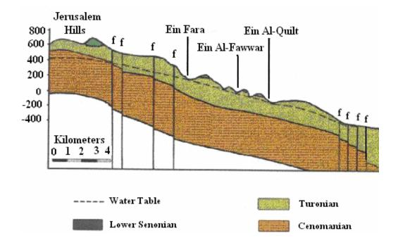
Figure 2.3: Geological sketch section along the line of springs in Al-Qilt catchment. (Abed Rabbo et. al, 1999).
